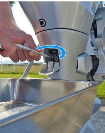
11. After draining the oil, install the drain bolt and new sealing washer, and tighten the bolt securely. Install the drain bolt cover.
