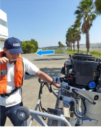
15. Remove the ACG cover. Wind the emergency starter rope (Refer to the Emergency starting procedure.) Drain the water from the cylinder by pulling the emergency starter rope several times.
