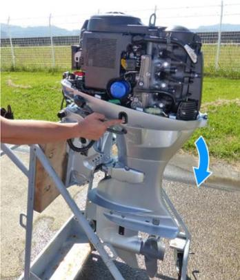
8. Tilt the outboard motor down.
