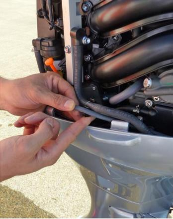
3. Release the drain tube from the projection of the intake manifold and bring the end of the drain tube out from beneath the cover.
