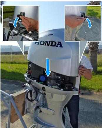
14. Leave the AC generator cover off and install the engine cover. Lock the engine cover fixing levers.
