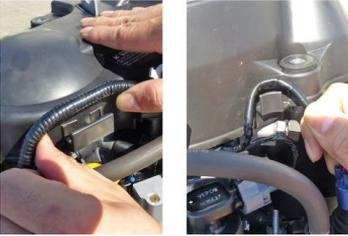
4. Remove the band clamp, harness and clamp bracket from the ACG cover. Then re-install on the engine side.
