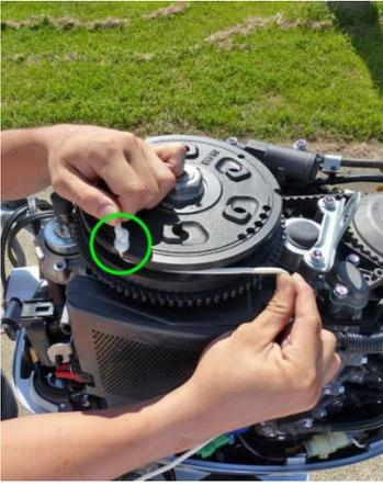
9. Set the knotted end of the emergency starter rope in the notch in the fly wheel.
