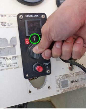
12. Turn the engine switch key to the ON position.
