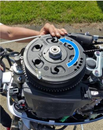
10. Wind the emergency starter rope clockwise 3 times around the fly wheel along the groove in the ACG rotor.
