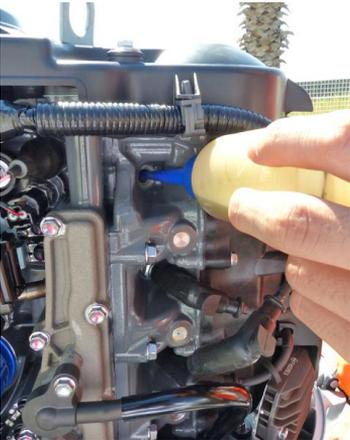
16. Pour a teaspoon of engine oil into all the spark plug holes.
