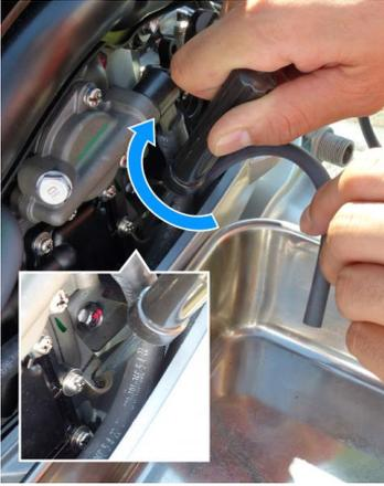
6. After draining, tighten the drain screw.
