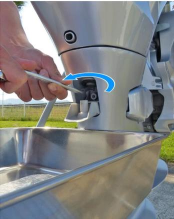
10. Place a suitable container under the oil drain guide, remove the drain bolt cover, engine oil drain bolt and washer. Drain the engine oil until the flow of old oil reduces to a trickle.
