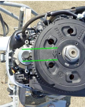
7. Turn the AC generator rotor anti-clockwise so that the arrow is lined up with the starter motor as shown.
